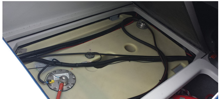
Figure 2. A ballast bag is pliable and collapsible, and often has two connected hoses in order to fill and drain the ballast (left). It was observed that the hoses could lift the drain connection above the lowest part of the ballast bag, resulting in a significant amount of residual water in the ballast bag (right). A hard ballast tank (bottom) fills an entire compartment, even when not full, and is generally inaccessible without tools. Photo credit: Tim Campbell.
