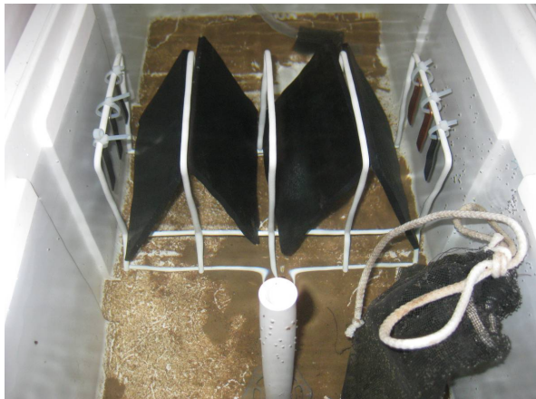
Figure 2. Inside of a settlement chamber showing a rack with four settlement plates and a mesh bag containing live adult mussels. Photograph by Renata Claudi.
