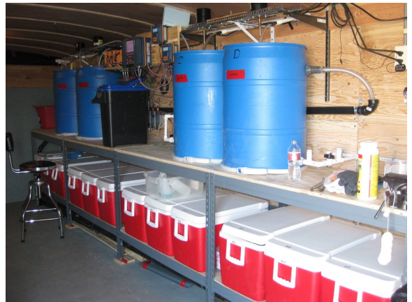
Figure 3. Complete laboratory set-up showing four mixing tanks (blue barrels), twelve settlement tanks (red coolers), and associated monitoring devices. Photograph by Renata Claudi.
