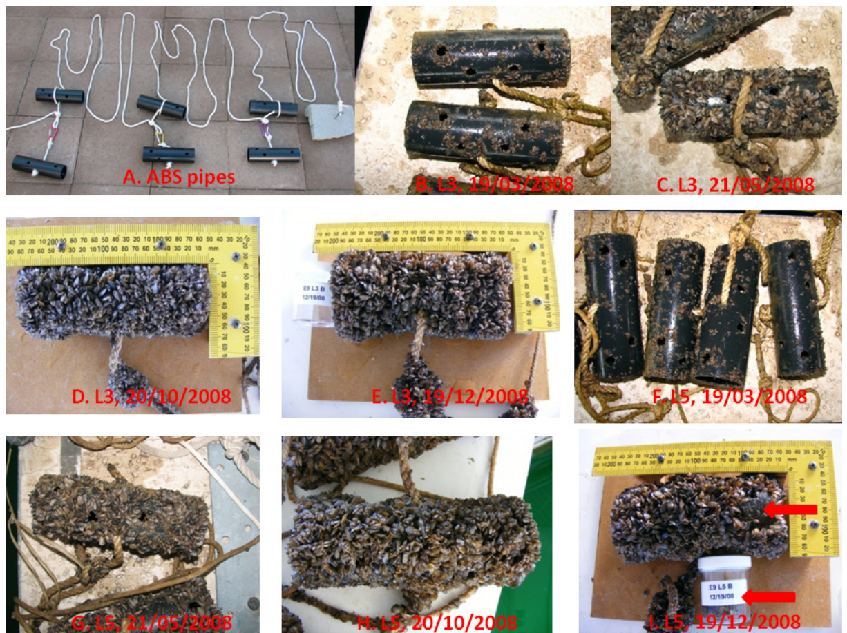
Figure 2. Colonization of quagga mussels on ABS pipes suspended in Lines 3 (L3: B-E) and 5 (L5: F-I). Photographs also demonstrate how the mussels were collected from each pipe: red arrows show where the mussels were taken from a measured area and transferred to a plastic bottle. Photographs by Wai Hing Wong.
