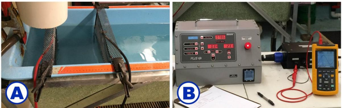
**Figure 2.** Electrified field exposure system consisting of a fiberglass exposure tank with iridium oxide-coated titanium mesh electrodes (A) and a Midwest Lake Electrofishing Systems Infinity Control Box<sup>®</sup> with a connected resistor box (B) (Photographs by James A. Luoma).
